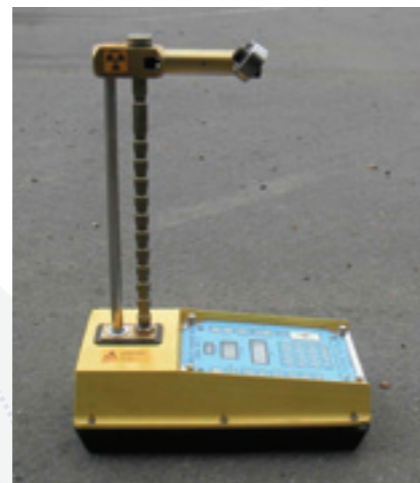
An NDM with the source assembly rod locked in the shielded position
