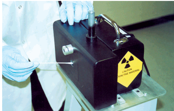
Using the NRL Wipe Test Kit on a caesium-137 source holder
